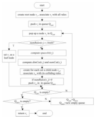
**Figure. 6** Flow-chart for implementation of D-Cuts. *binth* in the chart is a constant parameter defined as the maximum number of rules for leaf nodes. In D-Cuts, we set *binth*=8.
